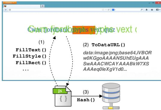
Figure 1: Canvas fingerprinting basic flow of operations
